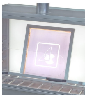
Light box behind to help in developing and washing the screens
