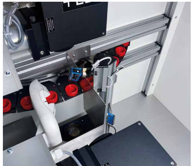
Application MOF MULTI Up to 4 marking positions at the same time on 1 component
