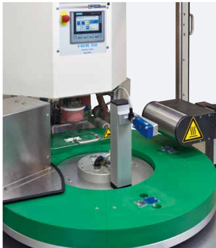
Multifunction jig surrounded by pad printing machine and components
