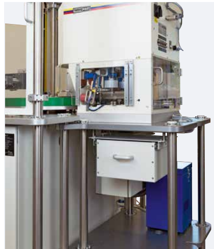
Assembly of satellite to rear side of machine with easy access to the printing units
