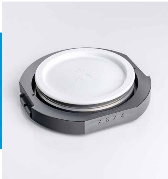
Ink refill without removing the doctor blade cup for short downtimes
