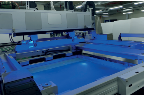
Blue LED light from top, camera from beneath checking the fiducial exposed in the screen.
