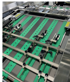
Even the sheet edge rollers will search for the correct position.
