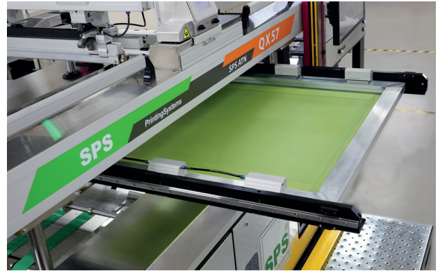
Simply slide the screen into the machine from the operator side.
