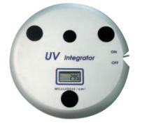
The amount of UV-energy required may vary to a large extent depending on the ink system (measurement values are based on the Kühnast UV-integrator).
