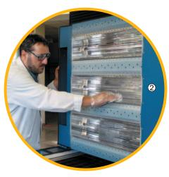
shades with a high content of clear varnish will require a little less curing energy than e.g. standard colour shades.
