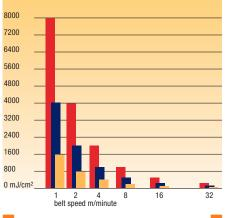
The relation of energy amount and the belt speed is inversely proportional. If speed is doubled efficiency will be half. The higher the initial efficiency the quicker you can cure.
