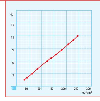
Comparison tests in our laboratory showed that the lamp output values measured with the Tesa/Hönle system are similar to those measured with the Kühnast integrator. With lower dosages the Tesa/Hönle system shows lower values than the Kühnast integrator and in a range of 200 mJ/cm<sup>2</sup> results of both systems are quite comparable.
