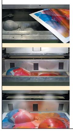
When first developing UV-curing inks formulation of an ink type suitable for deep drawing hardly seemed to be possible with such inks. The first UV-curing ink types had such a high cross-linkage that thermo-forming of prints was impossible. Only with development and combination of suitable photoinitiators combined with the appropriate resin systems and monomers UV-curing screen printing inks could be used for deep drawing of displays.
