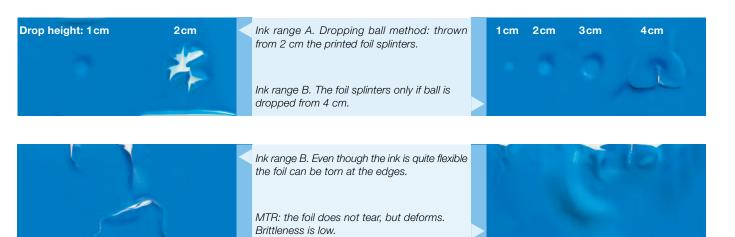
most interesting properties. At any rate that was the case with Musketeer MTR. Just think of substrates such as rigid PVC foils. Unfortunately, with these materials one often has the problem that the foil material becomes brittle when using rigid, highly cross-linking UV-inks. Sometimes even to such an extent that printed foils break or shatter like glass under low mechanical stress.
