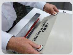
Press both buttons simultaneously to engage the clamping mechanism
