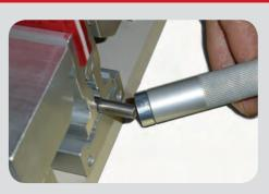
Place the set between the Qwik-Klamp jaws and press both buttons. With the clamps engaged, use the supplied magnet to remove the retaining pin. Then press either button to disengage the clamps and release the squeegee blade.
