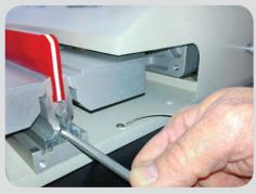
Insert the retaining pin and release the clamping mechanism by pressing either button
