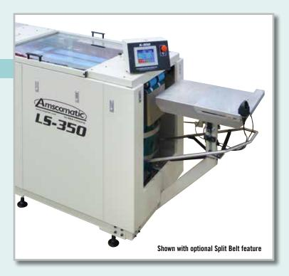
dual top belts with a gap that allows buttons, plackets, and zippers to pass through cleanly and smoothly.
