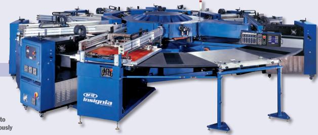
M&R's most aggressively priced multi-color UV system prints and cures up to six colors simultaneously. Since substrates don't need to be dried and stacked between colors, they don't have to be handled repeatedly. This prevents dimensional changes to substrates, and is especially beneficial for fragile substrates like glass. Since Insignia delivers finished prints in one revolution, it's possible to do color and registration adjustments for customer approval prior to the production run.
