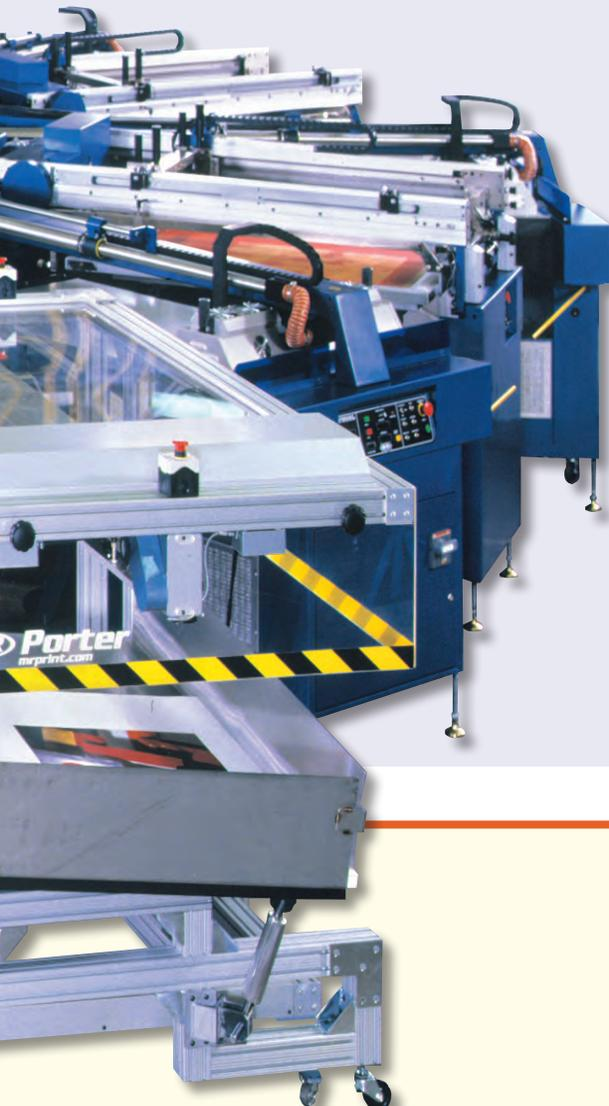
**M&R's versatile Conquest multi-color UV print/cure system simultaneously prints and cures up to six colors.**
