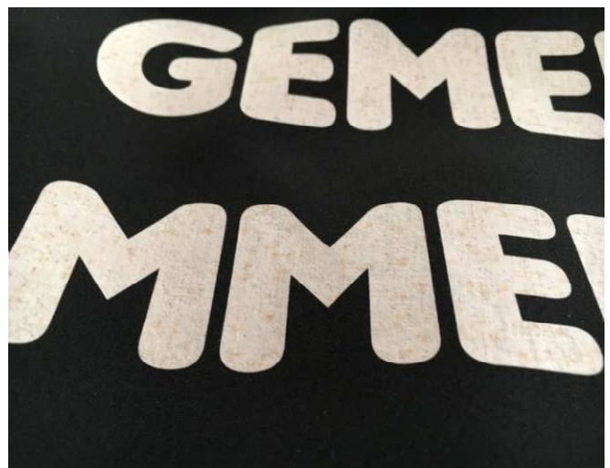
In the case of elastic fibers such as Lycra or Elastane, dispersion pigments dissolve from the fiber composite even at low temperatures.
