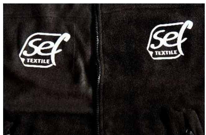
Left: a noticeable imprint is left with the standard parameters Right: no imprint when the transfer is made from the "rear"
