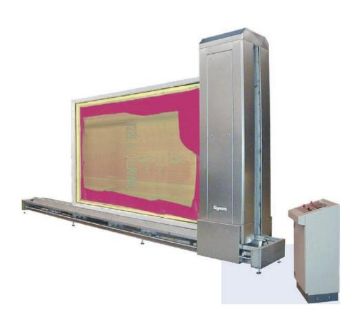
Linear developing tower with nozzle holders on both sides
