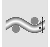
Mesh thickness D [ $\mu$ m] The mesh thickness D is measured according to ISO 5084. The tolerance is the defined range of the statistically ascertained mean values of mesh thickness.
