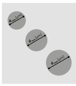
Thread diameter nominal  $d_{nom}$  [µm] The diameter  $d_{nom}$  is measured on the thread before weaving.
