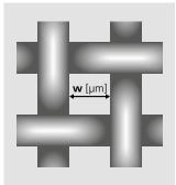
Mesh opening **w** [µm] The mesh opening **w** is the distance between two adjacent warp or weft threads.
