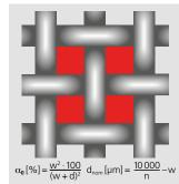
Percentage of open area  $\alpha_0$  [%] The percentage of open area  $\alpha_0$  is the sum of all mesh opening areas expressed as a percentage of the total screen area. It is calculated from the mean value of mesh openings and the actual diameter of the threads.
