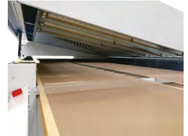
Infrared Lamps and upper section opening
