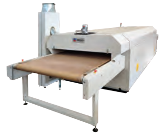
Exhaust fumes and outlet cooling hood
