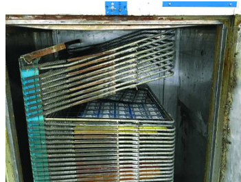
3. Dry the adhesive at below 80 °C
