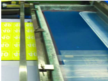
1. Print adhesive on the flock surface
