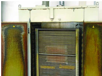
5. Cure adhesive according to manufacturer's instructions
