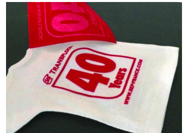
8. Peel carrier when cold, done!
