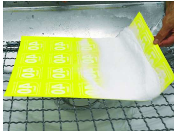
2. Apply hot-melt powder on the wet adhesive
