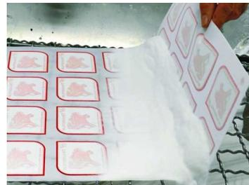
3. Apply hot-melt powder on the wet adhesive
