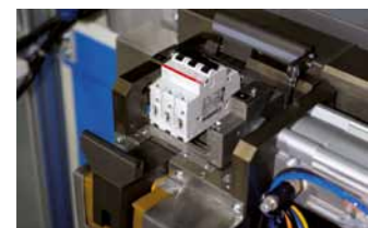
1. Detection: Number of circuit breakers
