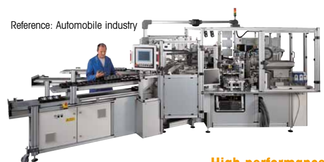
Ink surfaces – pad printing QR code – ink removal laser engraving
