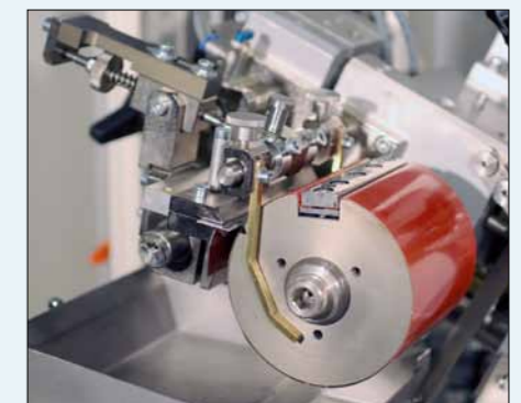
Fig.: Clamping cylinder mounted in rotary pad printing unit
